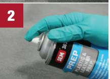
Apply Plastic & Leather Prep if needed. Scrub lightly with a nylon bristle brush to remove oil, grease and contaminants. Allow surface to dry, then vacuum.
