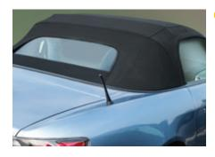
1 Additional flexibility is required when refinishing vinyl convertible tops with Color Coat. Mix 10 parts Color Coat toners to 1 part Super SEM Flex. Do not use Color Coat aerosols.
